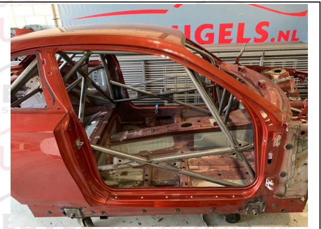
PHOTO 11 ANTI-INTRUSION DOORBAR – CO-DRIVER
